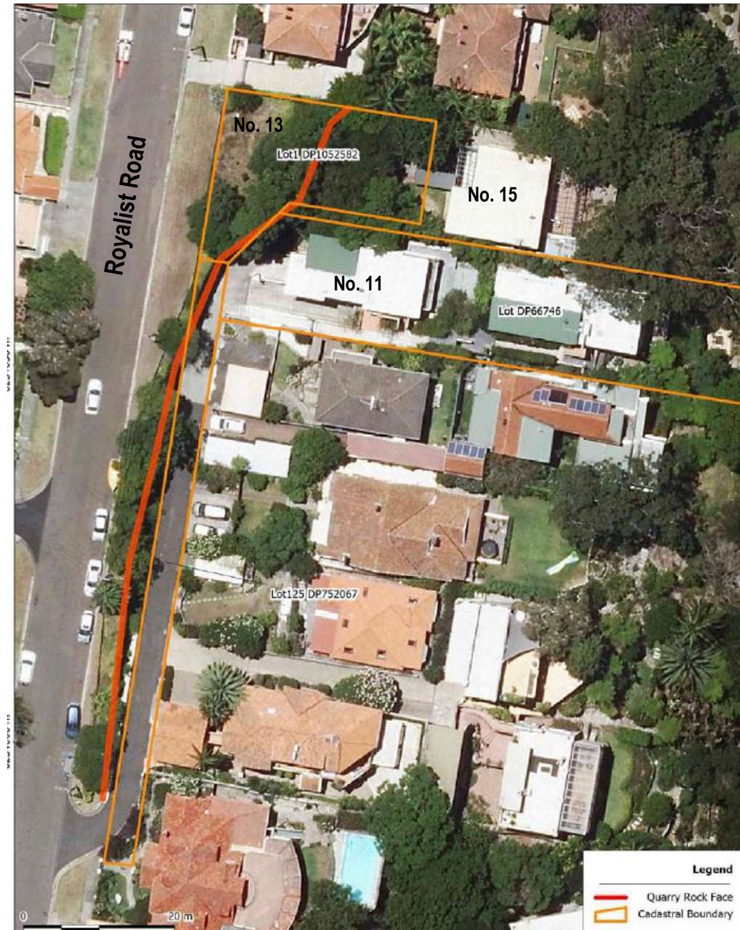
Extent of the excavated quarry wall within nos. 11, 13 and 15 Royalist Road, the accessway from Royalist Road to these properties and part of Royalist Road itself
