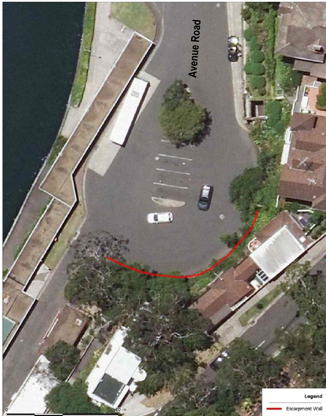
Extent of the excavated sandstone wall associated with the former tram terminus within the southern end of Avenue Road
