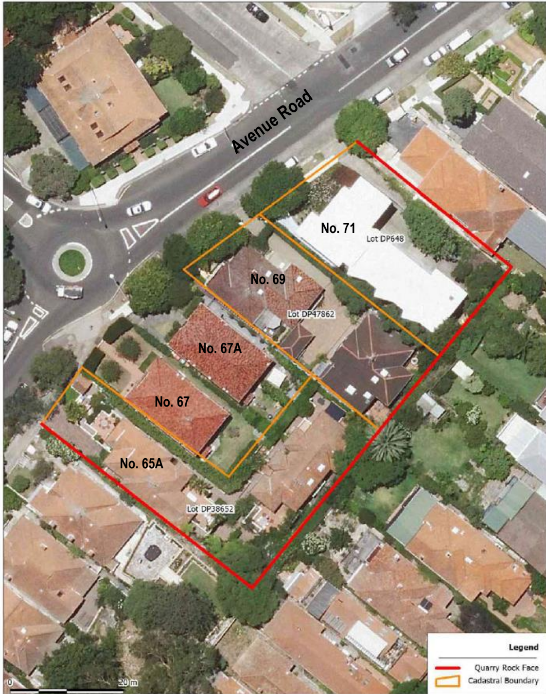
Extent of the excavated quarry wall within nos. 65A, 69 and 71 Avenue Road
